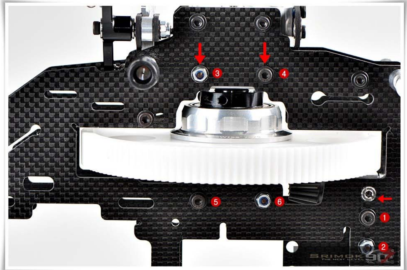
Picture C: Push middle Main Bearing Block down abut lightly
