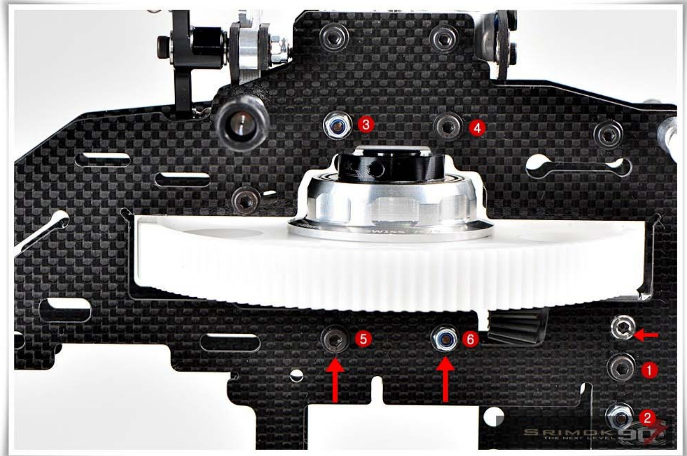
Picture D: Push lower Main Bearing Block abut tightly
